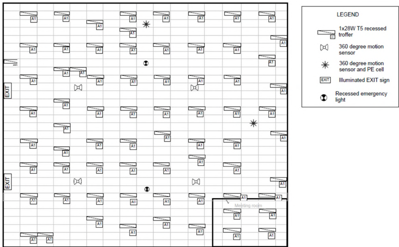
Figure 14: Sample RCP for Aggregate Method 1 – Example 1
