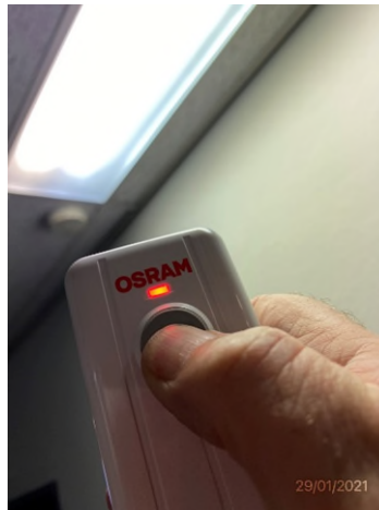
Figure 20: Photograph showing ballast discriminator test
