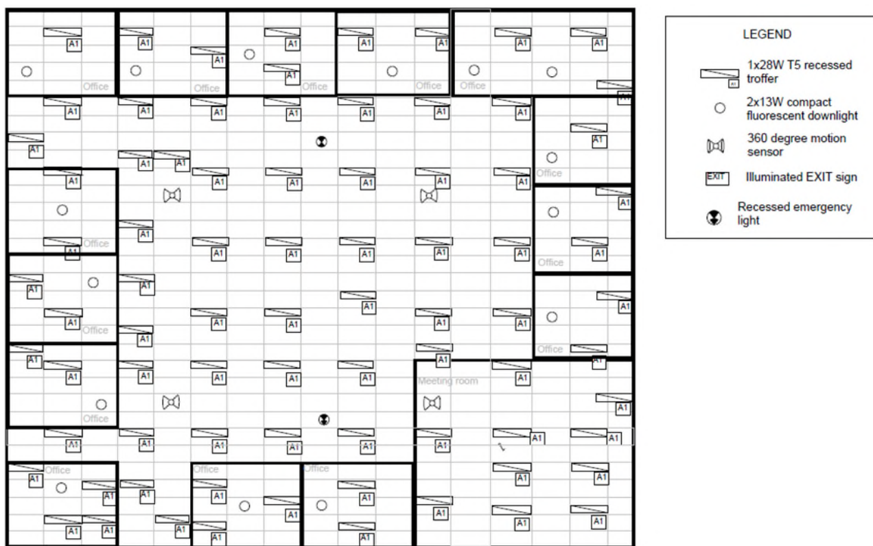
Figure 16: Sample RCP for Aggregate Method 2 example 1
