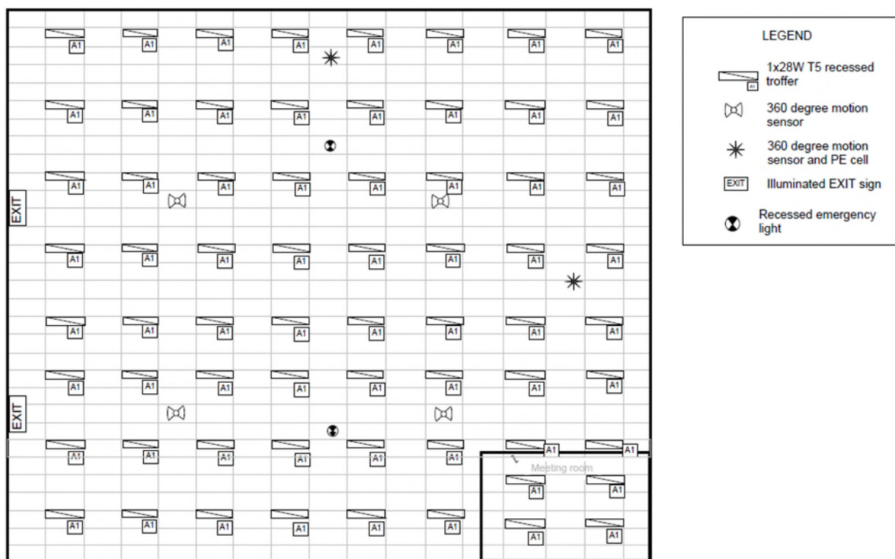
Figure 8: Sample RCP for Grid Method – Example 1
