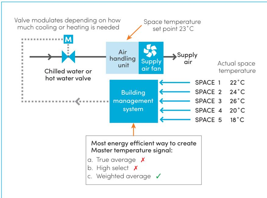
**Figure 5: Control strategies to generate a master air handling unit supply air temperature signal**
