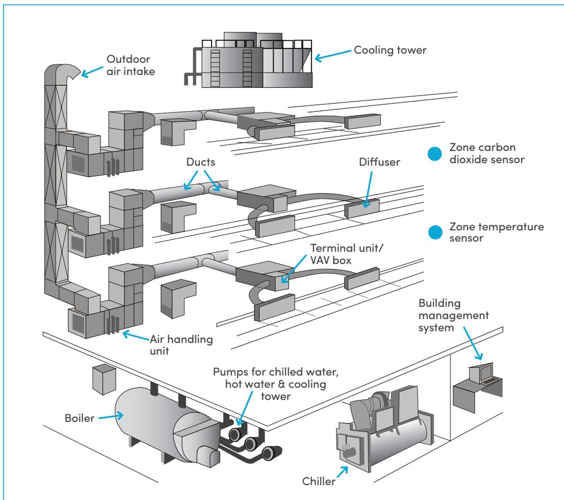
**Figure 1: Main components of a typical commercial HVAC system**
