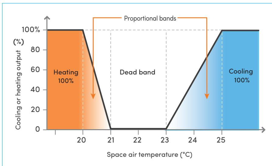
**Figure 4: Typical energy efficiency temperature set point and control bands**
