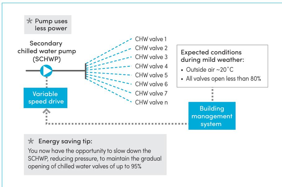
**Figure 17: Minimised pumping energy at SCHW loop - Operation of HVAC system under part-load conditions**
