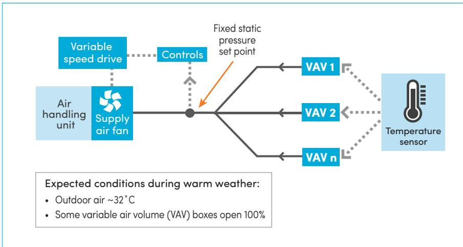
**Figure 8: Variable air volume air distribution under full-load (typical summer peak) conditions**
