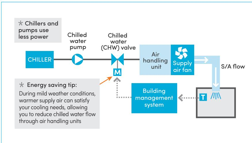
**Figure 6: Opportunity for supply air temperature reset – constant air volume system**
