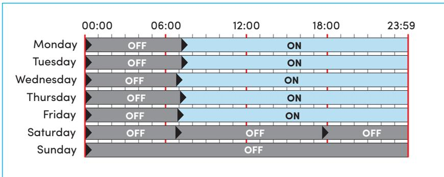
**Figure 2: Fixed time schedule for HVAC system on a building management system**
