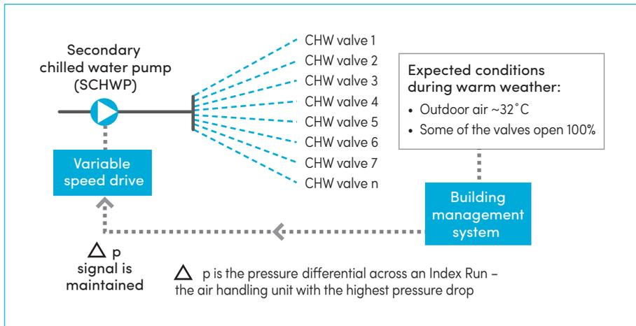
**Figure 16: Minimised pumping energy at secondary chilled water loop – operation of HVAC system under full-load (typical summer peak) conditions**
