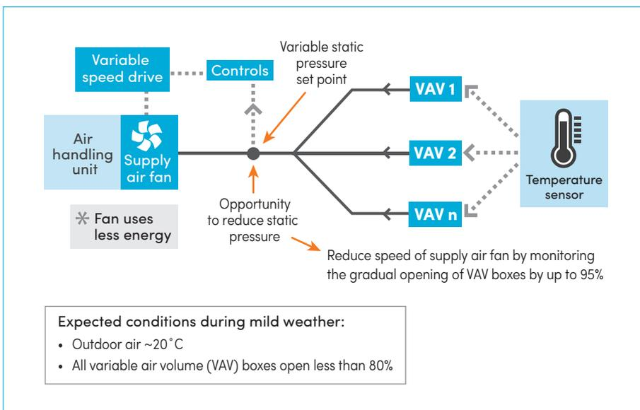
**Figure 9: Variable air volume air distribution under part-load conditions**
