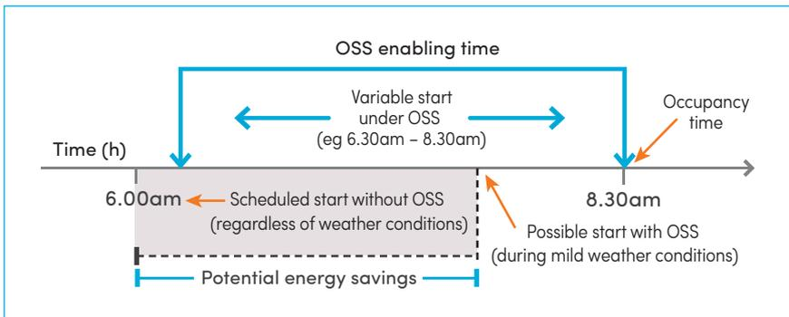
**Figure 3: Potential energy savings of optimum start**
