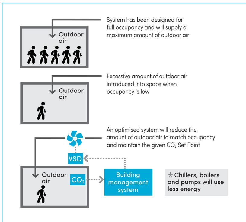
**Figure 14: Demand control ventilation of spaces with variable occupancy**
