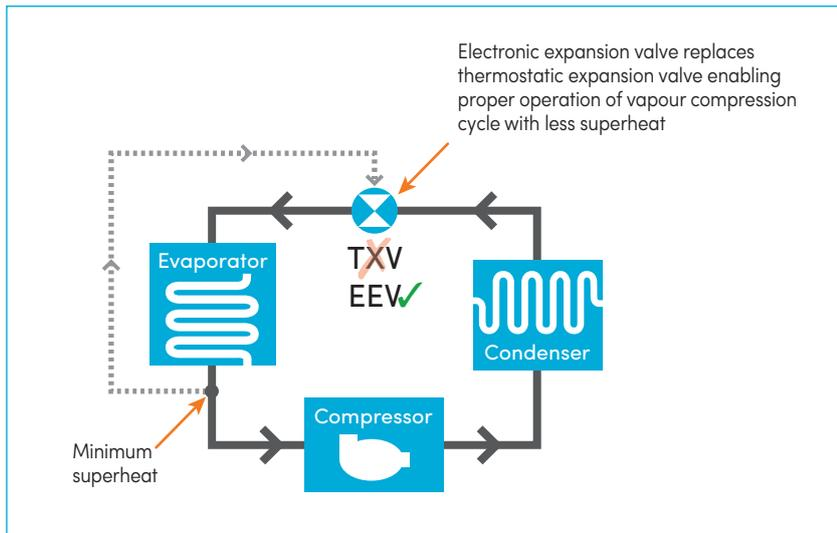
**Figure 11: Thermostatic expansion valve is replaced with an electronic expansion valve**
