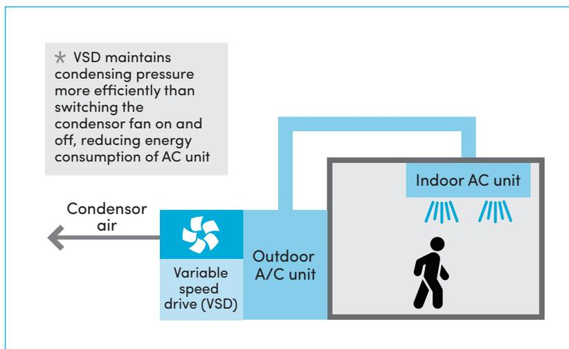
**Figure 18: Condensing pressure of a split air conditioning unit maintained by a variable speed drive controller**
