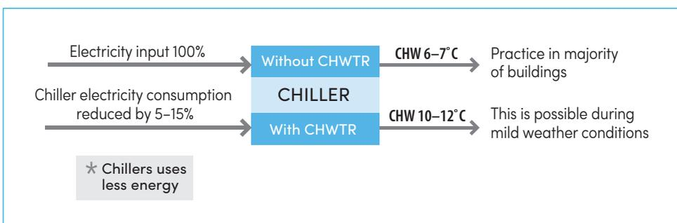
**Figure 10: Benefits from higher chilled water temperature (chilled water temperature reset)**
