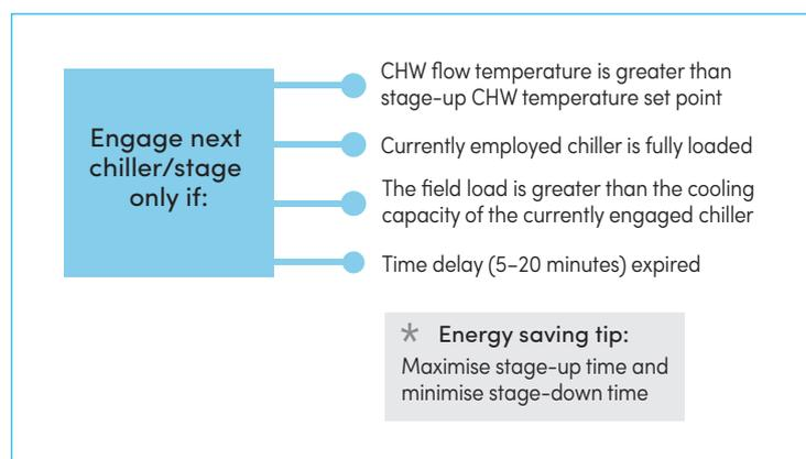
Figure 7: Chiller staging logic
