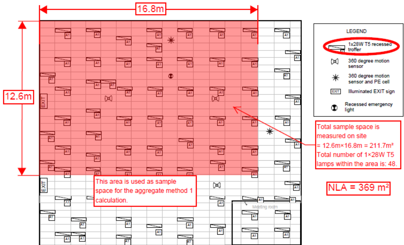
Figure 14: Sample marked up RCP for Aggregate Method 1
